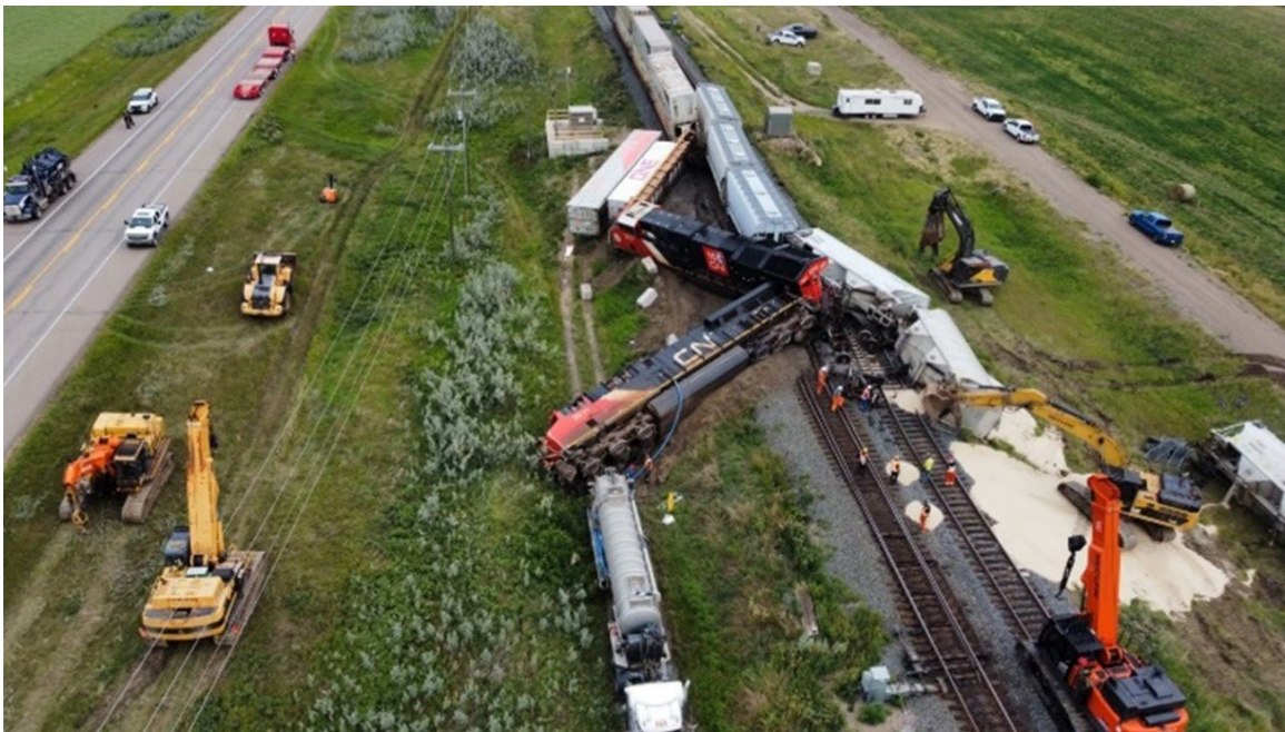
Figure 3. Derailed rolling stock after the collision, looking east (Source: Canadian National)
