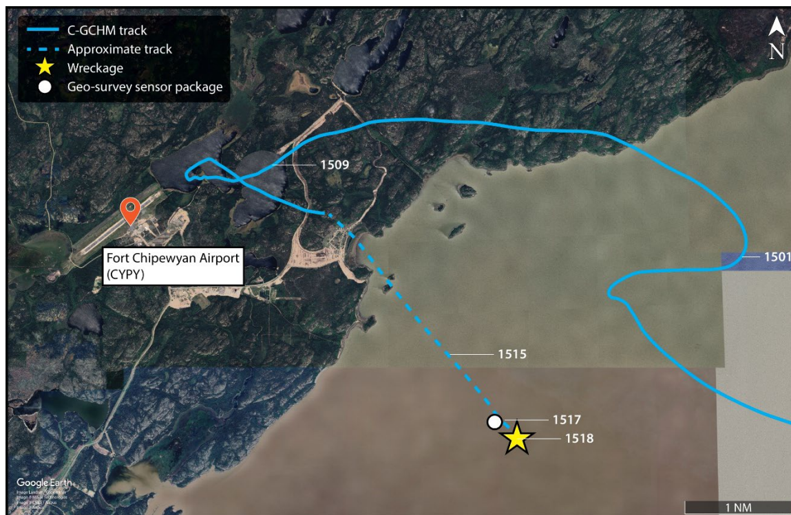
Figure 2. Composite depiction of the final minutes of the occurrence flight, based on available data with times and the approximate track (Source: Google Earth, with TSB annotations)
