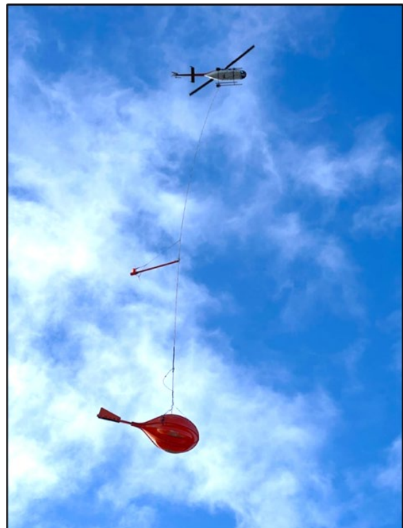
Figure 1. A Bell 206L helicopter with 300-foot longline and geo-survey sensor (bird) (Source: Hanley Heli Service Inc.)
