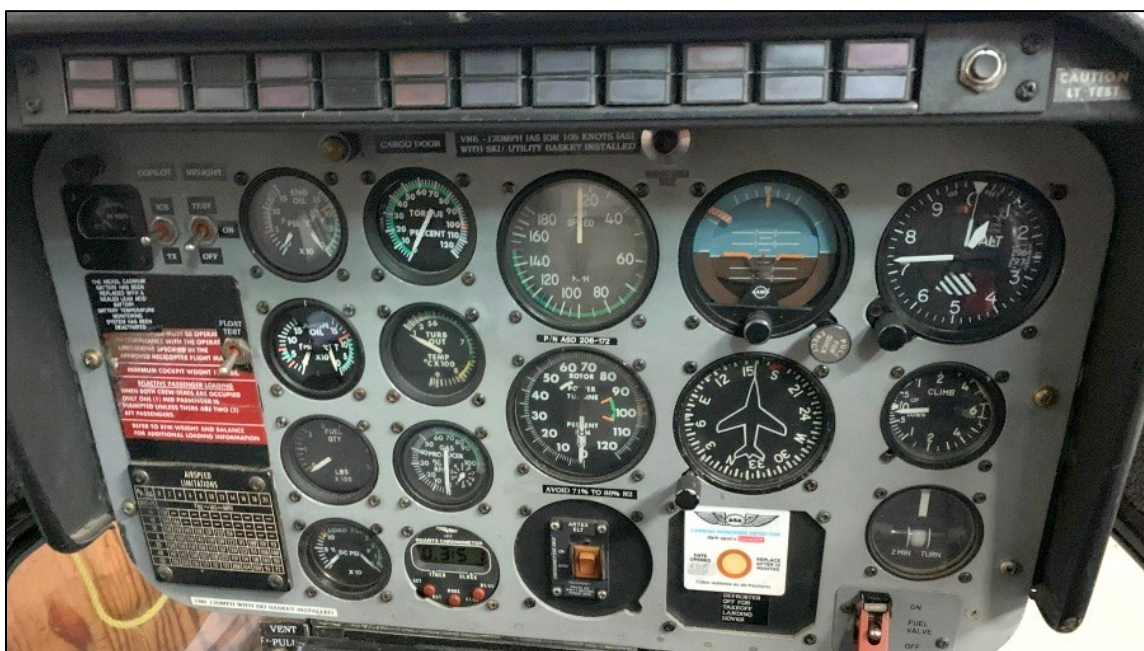
Figure 4. The occurrence helicopter’s instrument panel, configured in the standard “T” format (Source: Third party, with permission)
