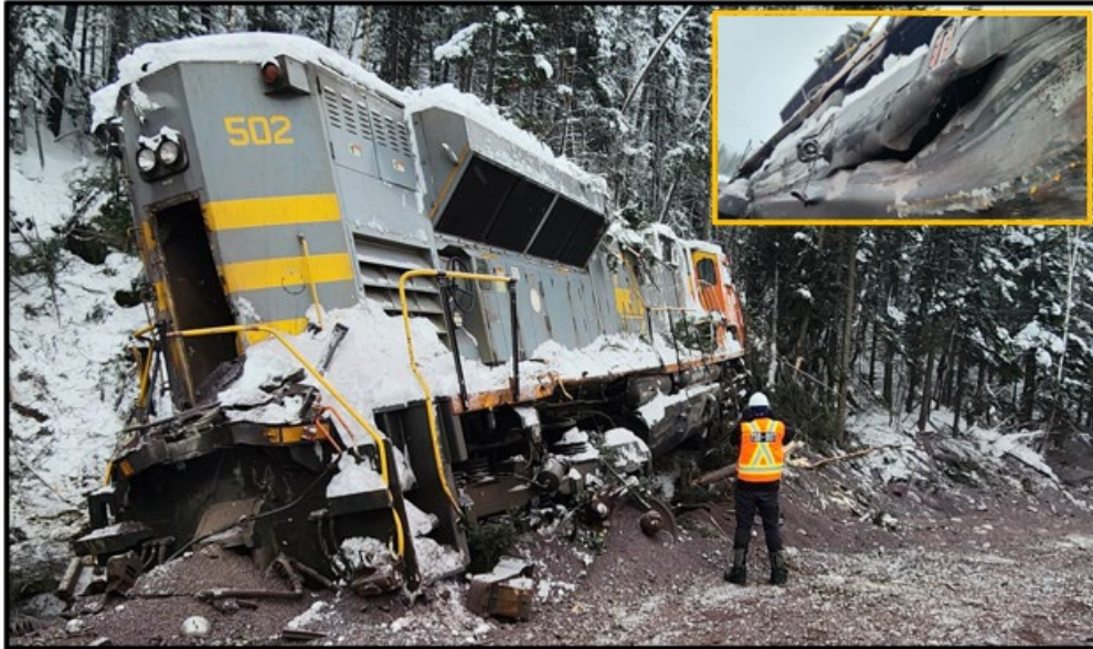
Figure 3. Derailed locomotive QNSL 502 with inset showing its punctured fuel tank (Source of main image: TSB. Source of inset image: TSB)
