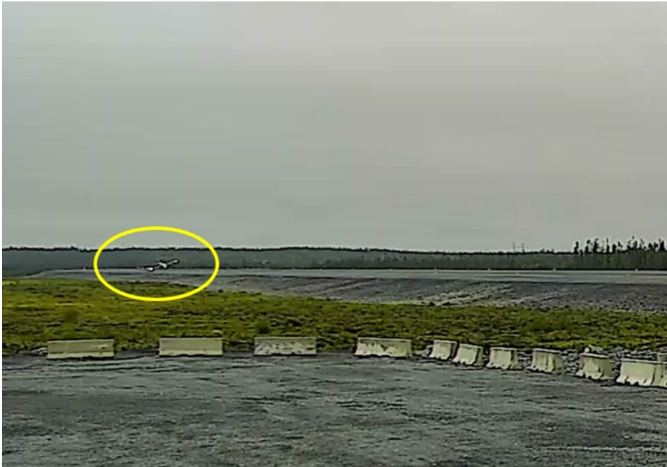
Figure 2. Occurrence aircraft impacting the runway (Source: Third party with permission and with TSB annotations)
