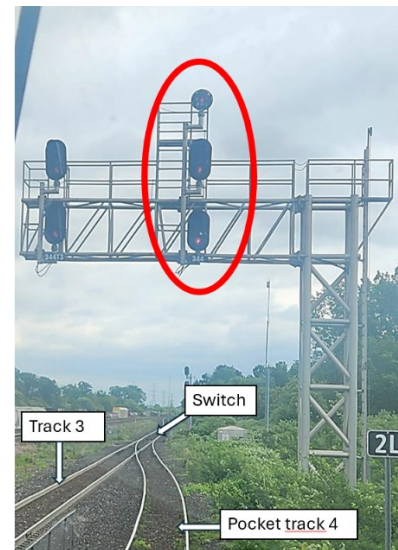
Figure 3. View of high-mast, 3-aspect signal 344 displaying a Stop indication, looking eastward from pocket track 4 at Aldershot (Source: TSB, photo taken post-occurrence)
