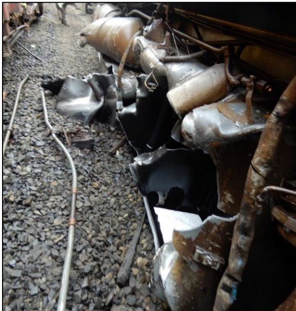
Figure 4. Severely damaged fuel tank on the lead locomotive of train 804 (Source: TSB)
