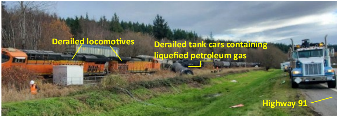
Figure 3. Derailed rolling stock after the collision (Source: TSB)
