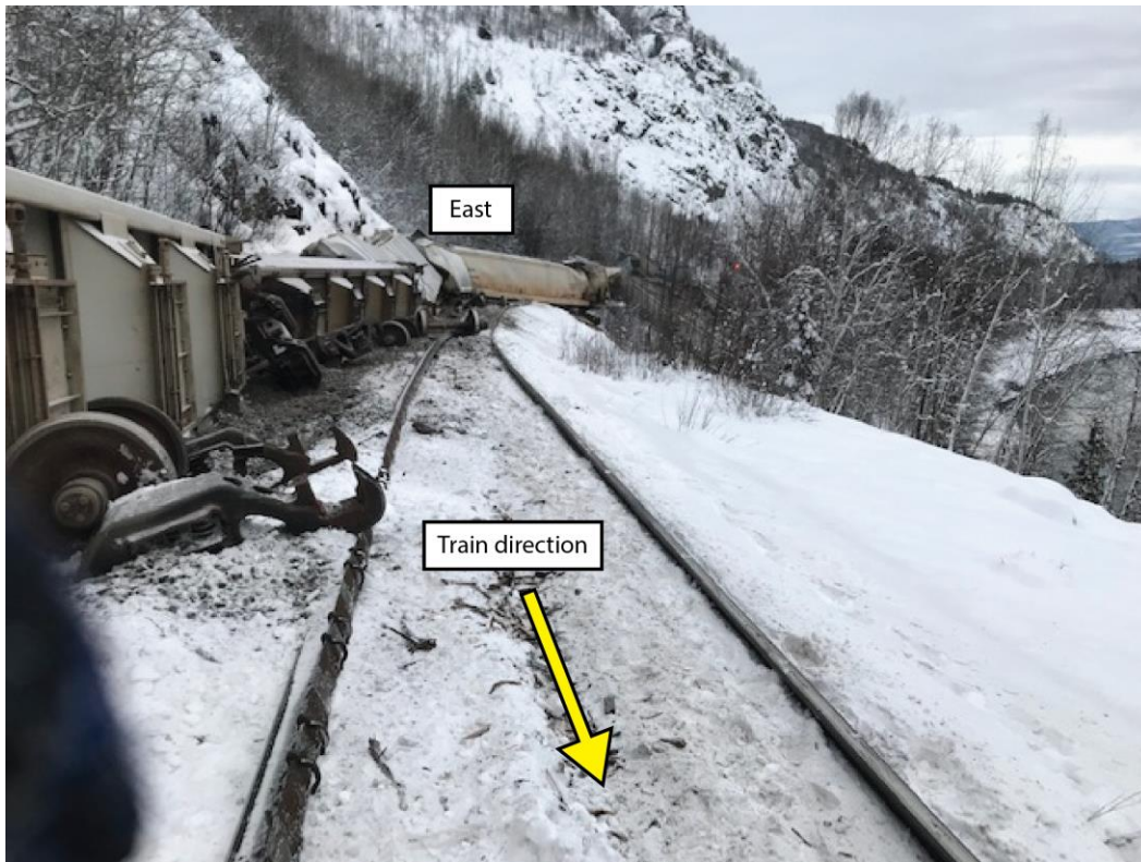
Figure 2. Derailed cars to the high (north) side of the eastern spiral of the 6-degree left-hand compound curve, looking east (Source: Canadian National Railway Company, with TSB annotations)
