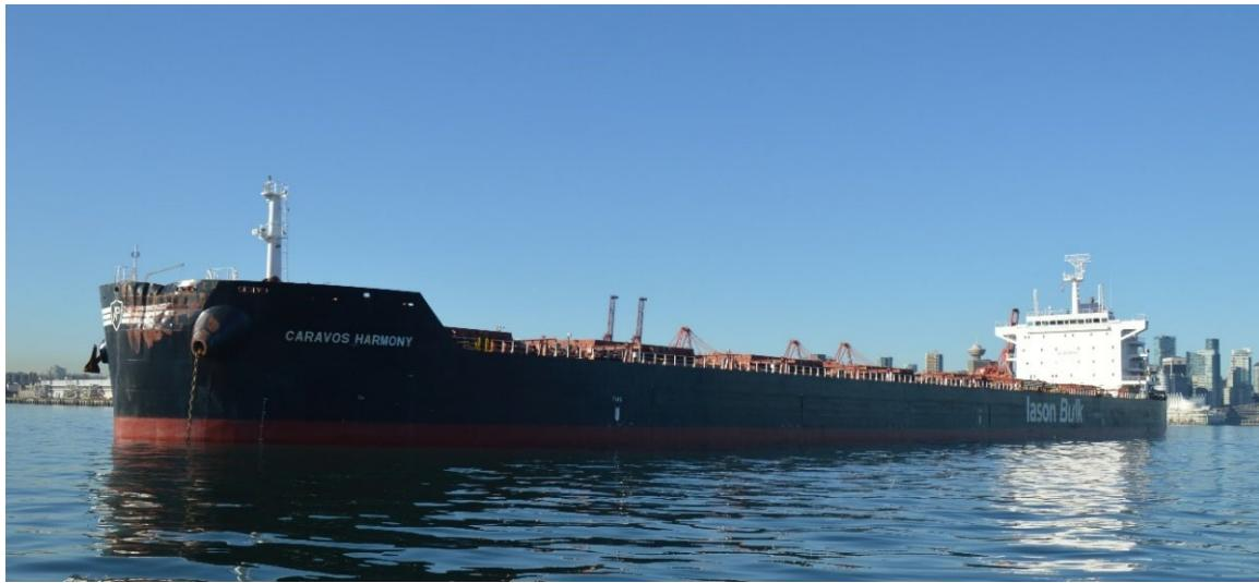
The vessel has 2 anchors, 1 on either side of the bow. Each anchor chain is restrained by a chain stopper and controlled by a windlass, and each windlass has a manual brake and gear that must be released in order to deploy the anchor. The vessel is not fitted with a bow thruster.
