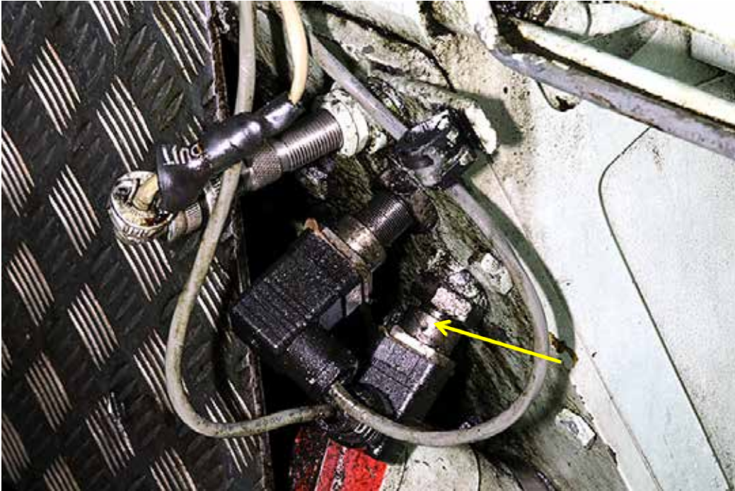
Close-up of governor and overspeed sensors. The yellow arrow shows the orientation of the 22% overspeed sensor index hole.
