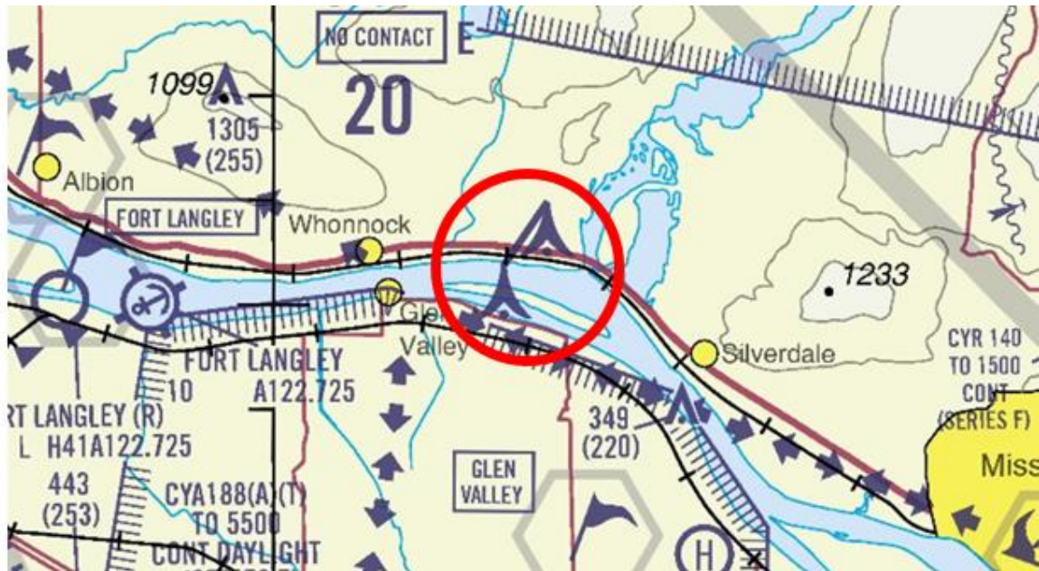
Figure 3. Visual flight rules navigational chart for the area. The power lines crossing the Fraser River are circled. (Source: NAV CANADA, with TSB annotations)
