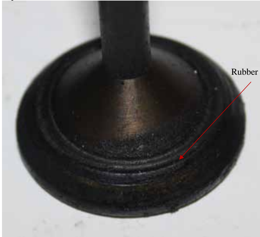
(b) Close-up view of the rubber seal
