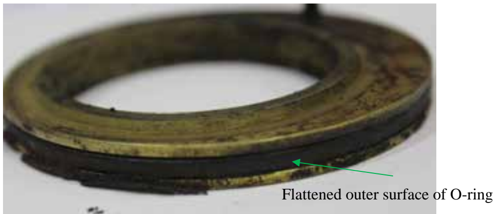
Figure 9: Side view of the seat ring showing the excessive wear on the O-ring of the main reservoir check valve from locomotive unit CEFX-3166
