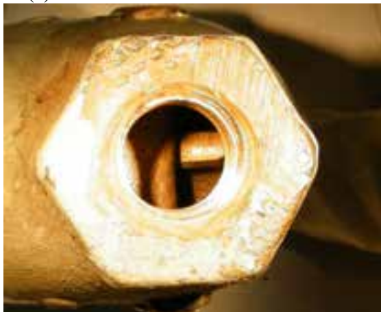
(b) Inside view of the valve from the entrance hole after removal of the inlet pipe
