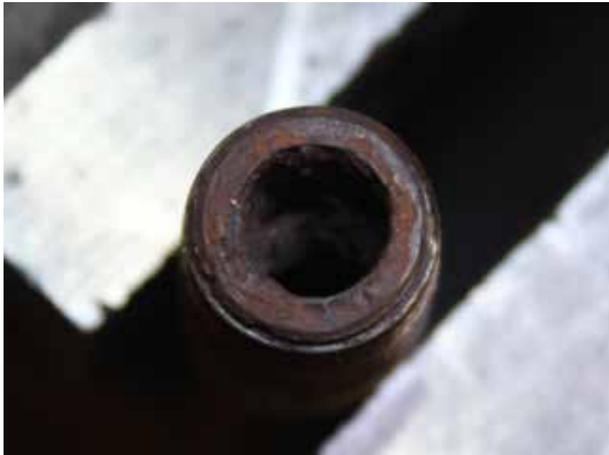
Figure 11: Photo showing the rusty end of the outlet pipe of the dead engine pressure regulating valve from locomotive unit CEFX-3166
