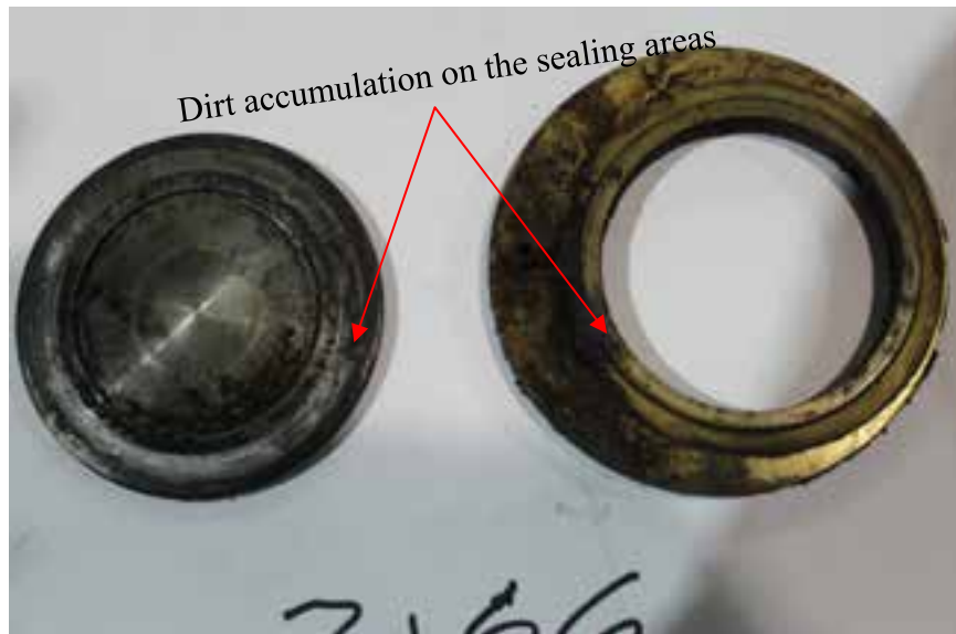
Figure 8: Significant dirt accumulation on sealing areas of both disc and seat ring of the main reservoir check valve from locomotive unit CEFX-3166
