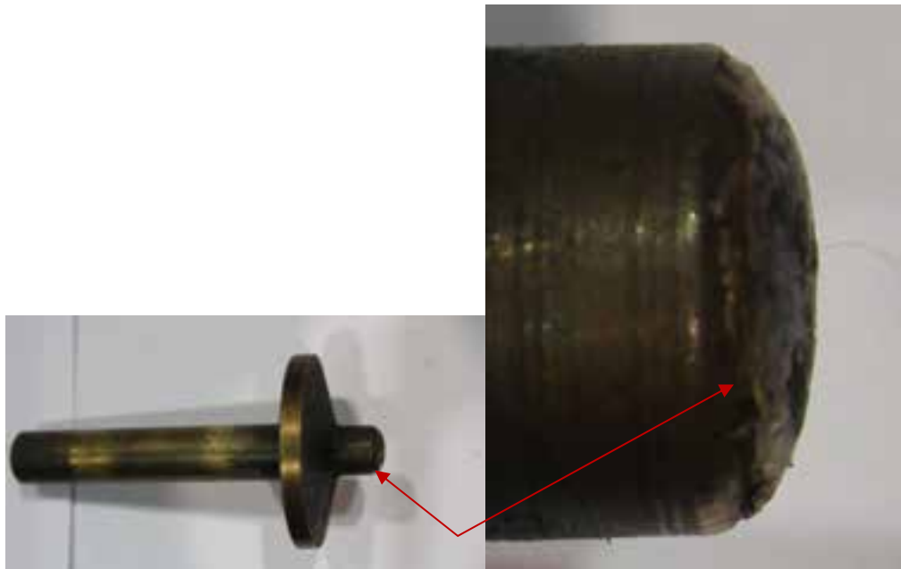
Figure 20: Photo of the QR valve lifter showing the damage to the head (see arrows)
