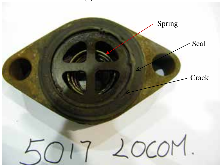
(b) Outlet side of the valve
