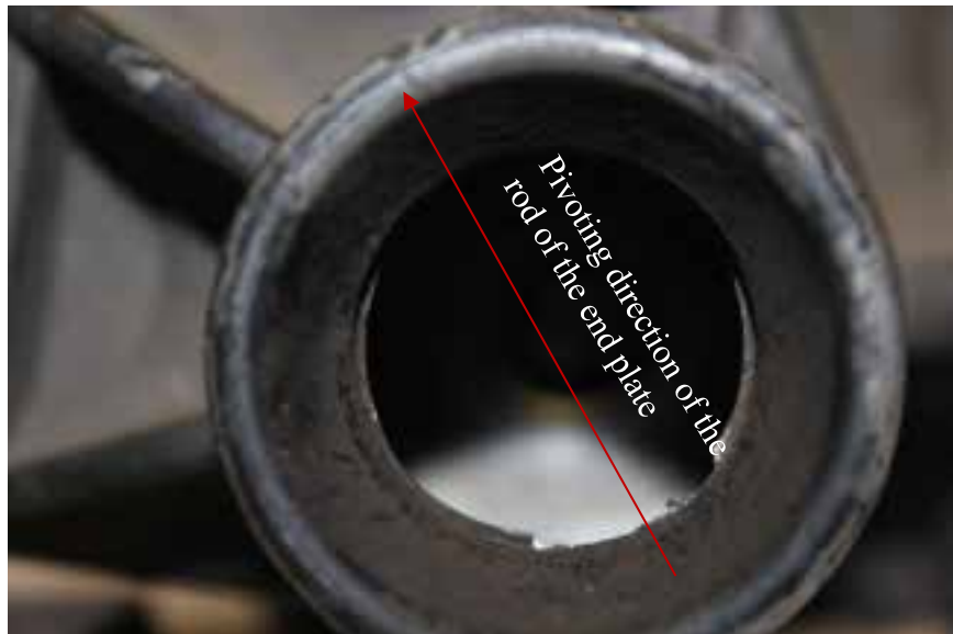
Figure 18: Damage on the edge of retaining hole for the end plate on the QRB valve's body
