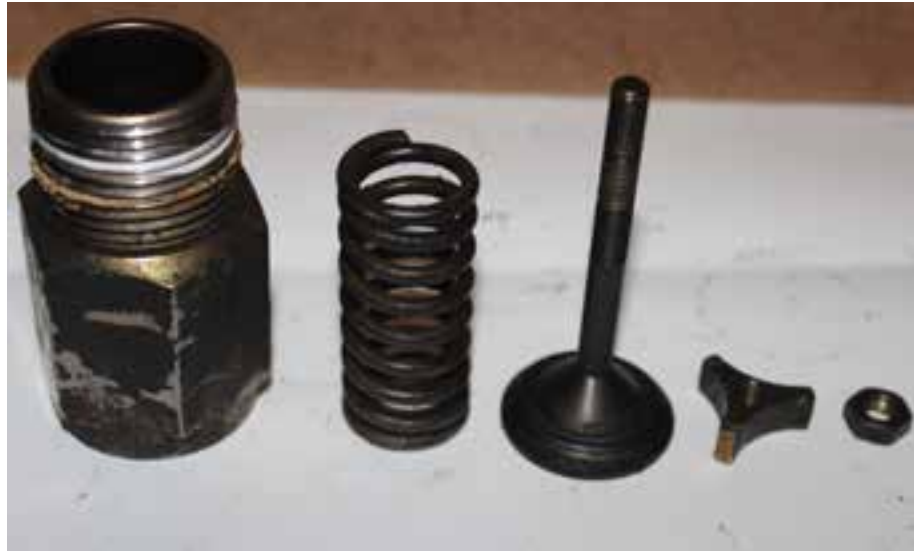
(a) Components of disassembled relief valve
