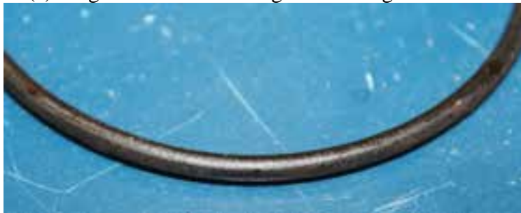
(b) O-ring between the seat ring and the housing body of the check valve
