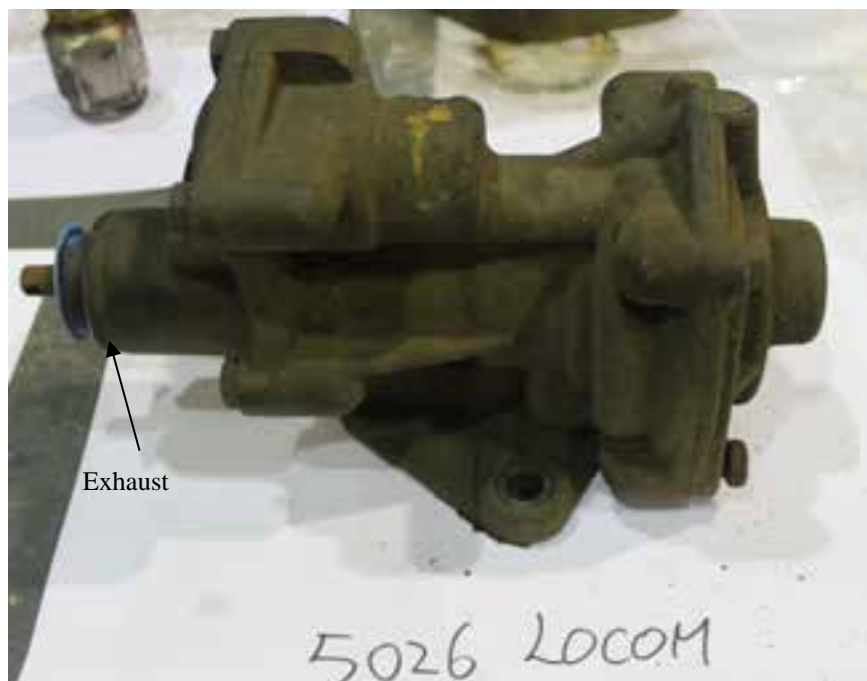
Figure 16: Photo showing the retrieved QRB valve from locomotive unit MMA-5026
