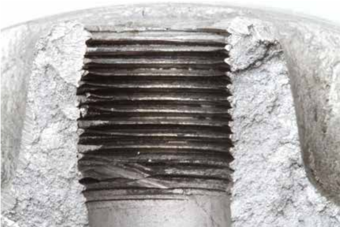
Figure 44: Mounting bolt thread damage in separated portion of cam bearing Note the thread damage is localized at the fracture edges
