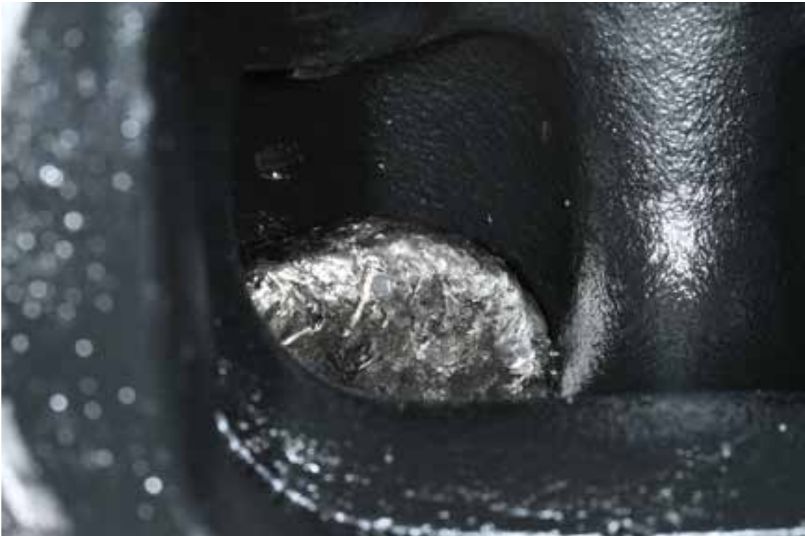
Figure 22: Exhaust valve head jammed in exhaust port
