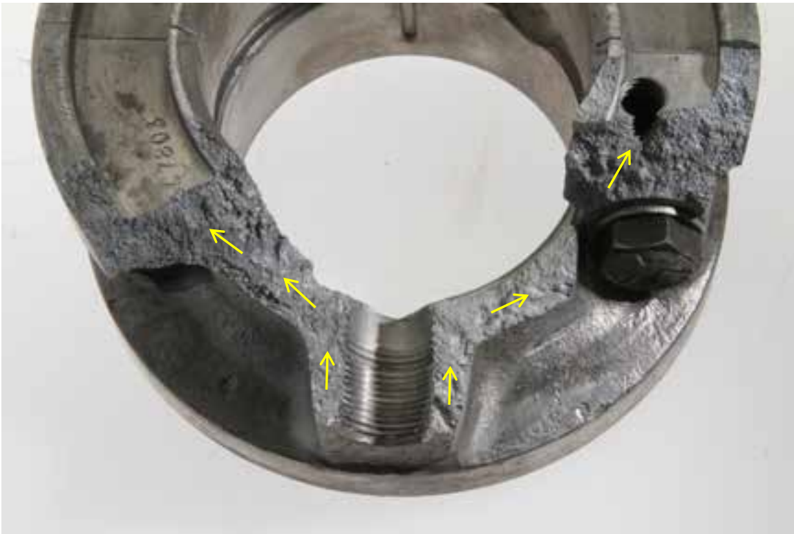
Figure 43: Cam bearing showing direction of fracture (arrowed)
