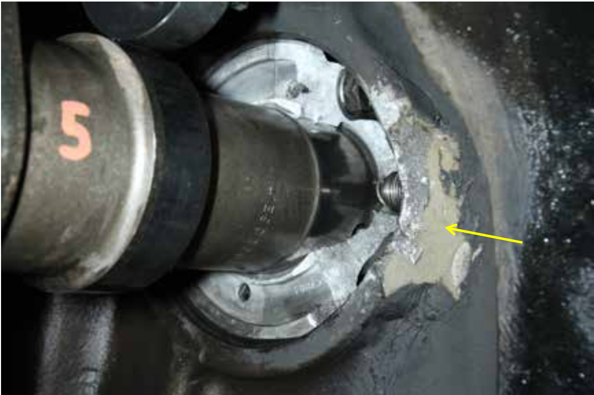
Figure 36: R4/R5 cam bearing bore showing previous repair (arrowed)
