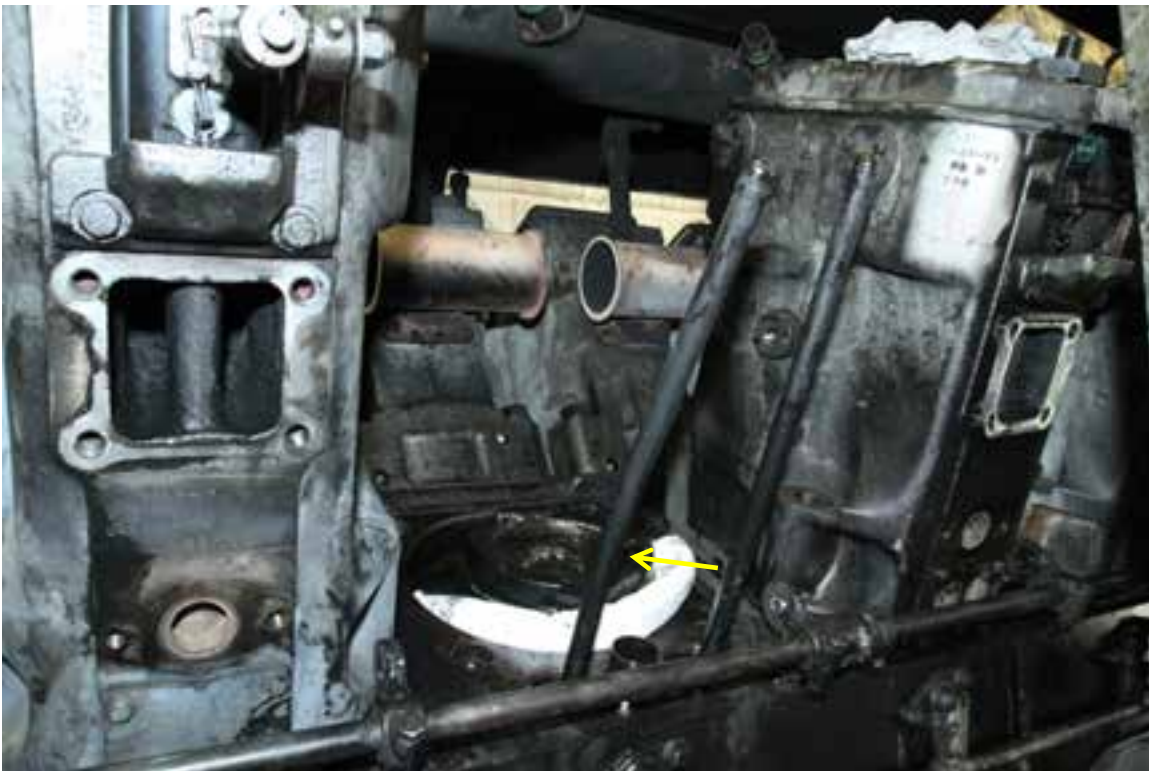
Figure 20: Bent PA R5 intake pushrod (arrowed)
