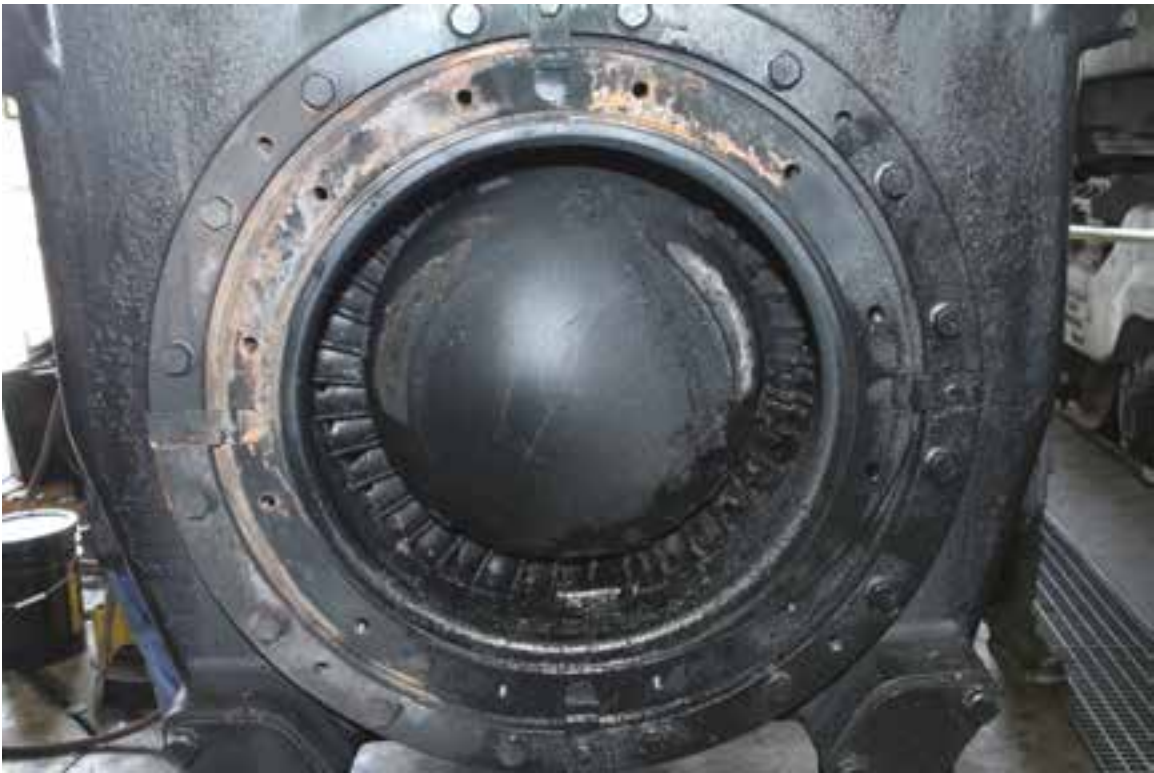
Figure 27: Turbocharger being removed from MMA 5017 Note buildup of coked oil
