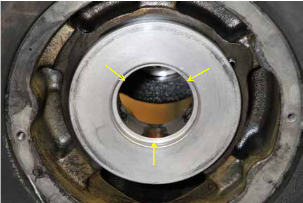
Figure 30: Compressor bearing showing damaged areas (arrowed)
