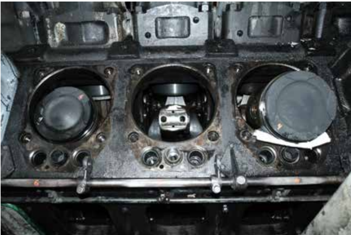
Figure 24: Pistons R6 (left) and R4 (right) showing crown colour and condition
