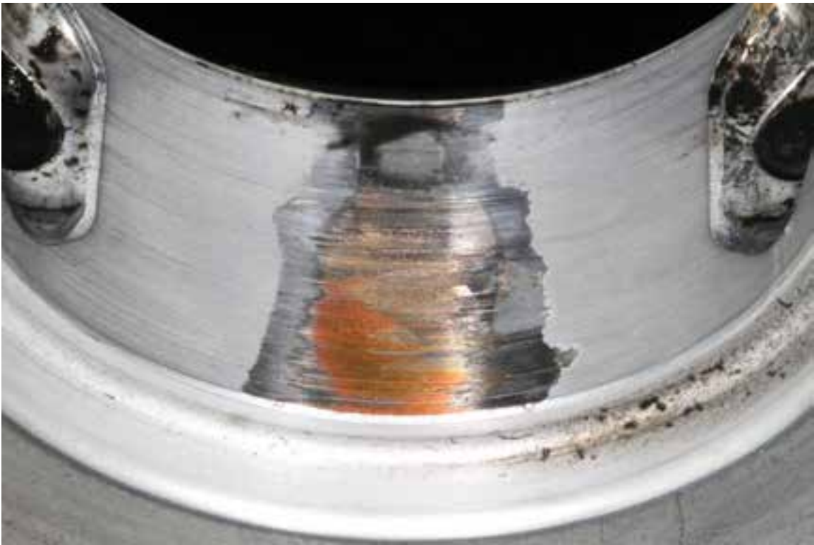
Figure 31: Close-up of compressor bearing damage
