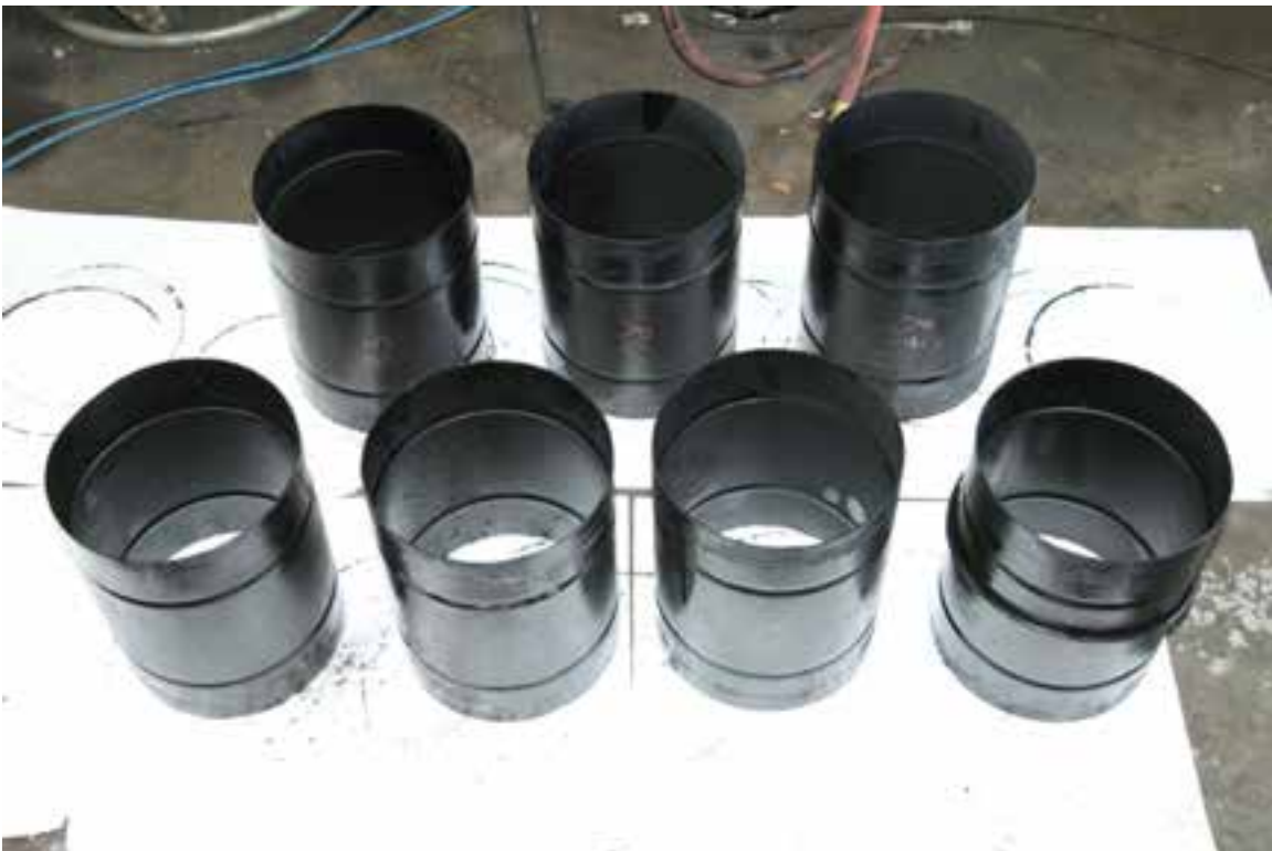
Figure 8: Right side intake manifold tube sections showing oil buildup
