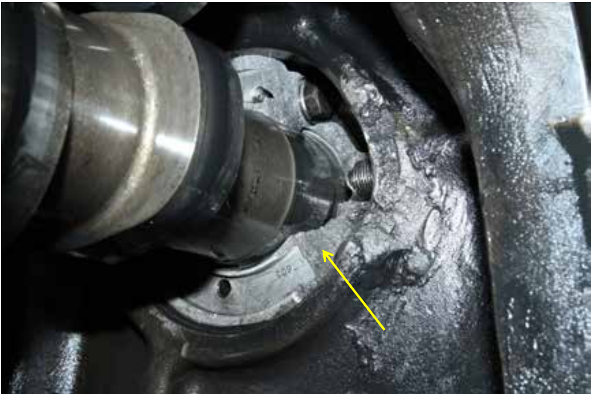
Figure 6: Broken camshaft bearing between PA R4 and R5 (arrowed)
