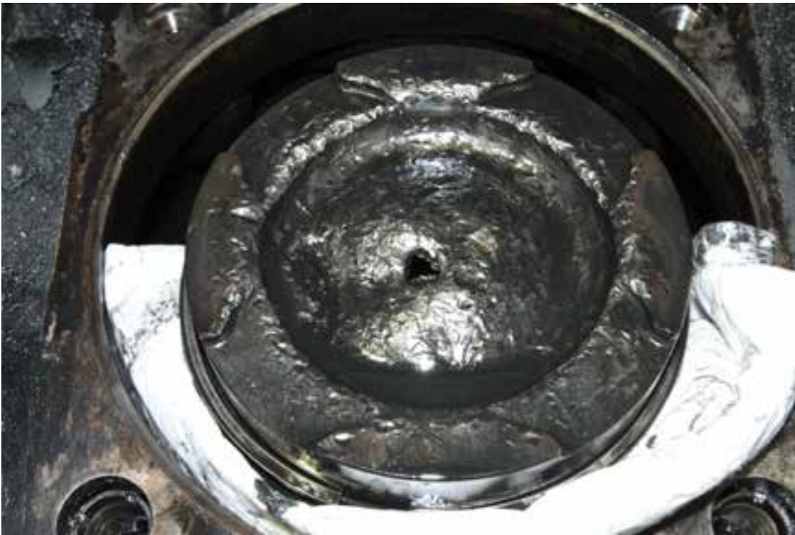
Figure 19: Piston crown of PA R5 Note the valve stem sized hole and oil puddle
