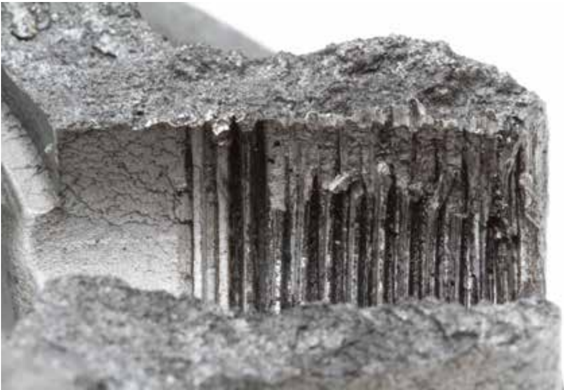
Figure 47: Mounting bolt thread damage in remaining portion of cam bearing Note the thread damage is localized at the fracture edges.
