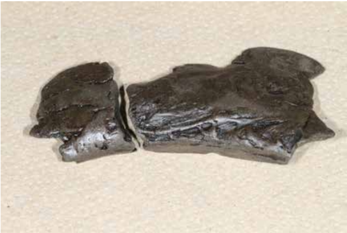
Figure 37: Recovered section of cam bearing bore repair material
