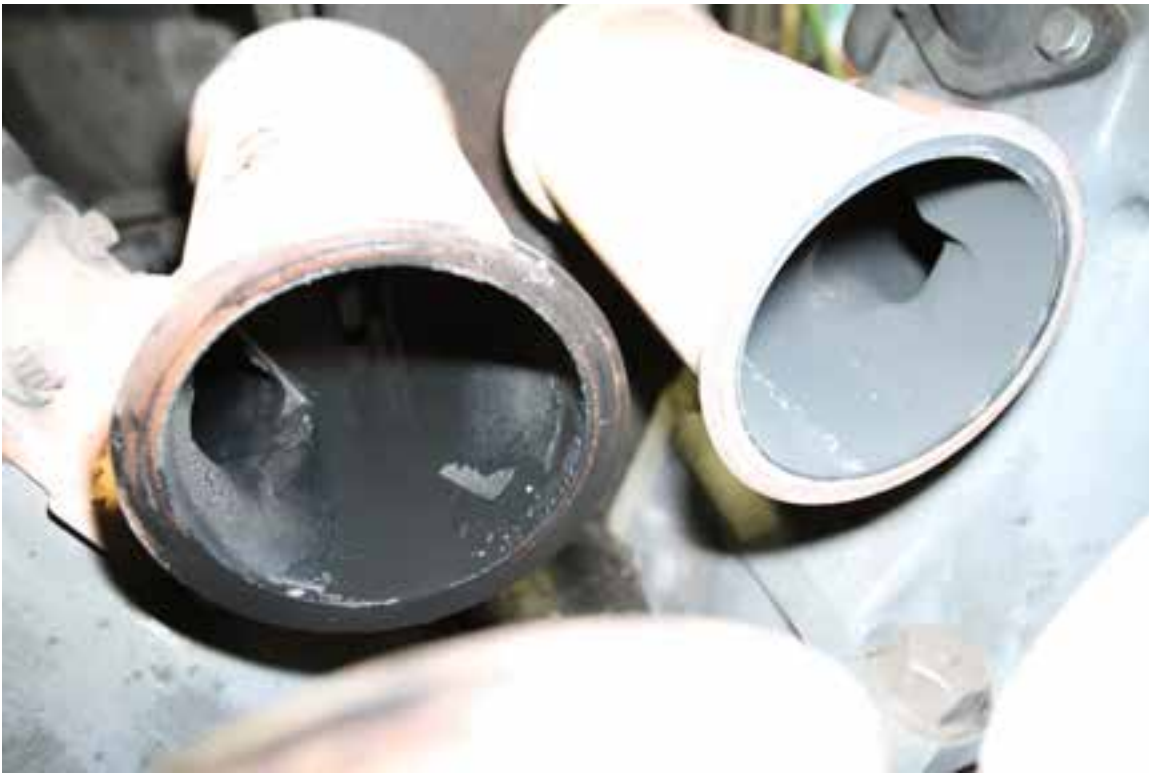
Figure 11: Exhaust manifold bodies for cylinders R8 and L8 showing oil buildup
