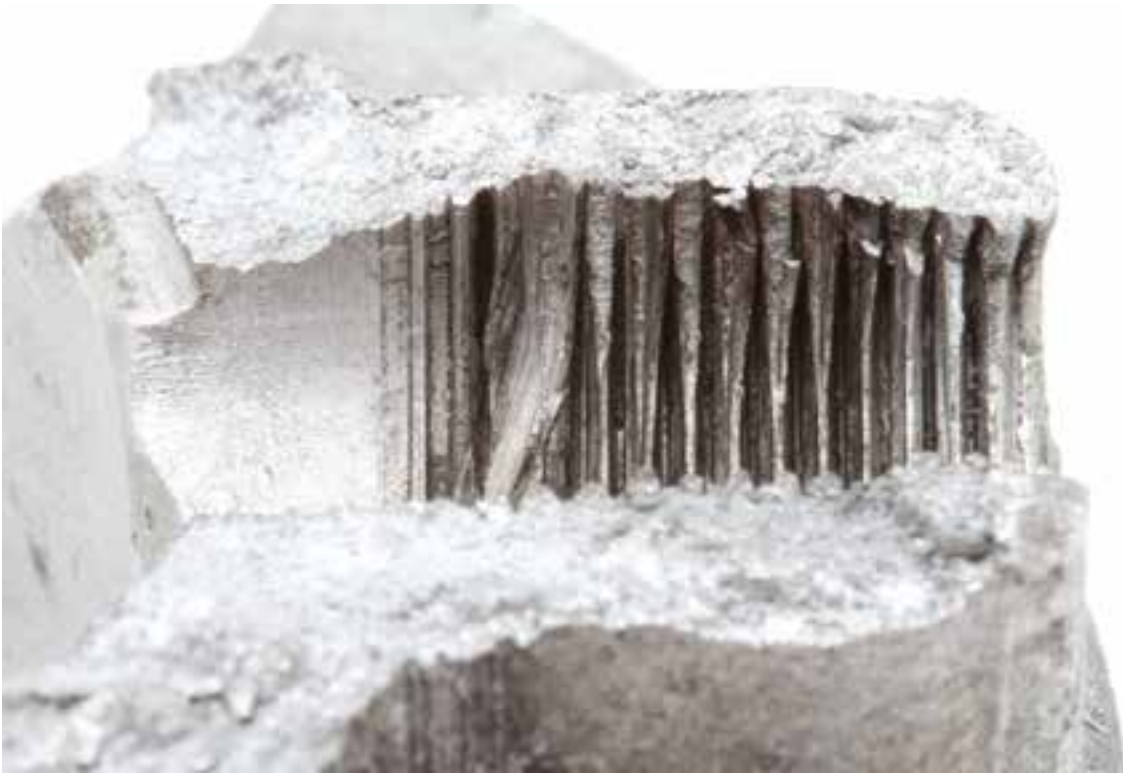
Figure 45: Mounting bolt thread damage in separated portion of cam bearing Note the thread damage is localized at the fracture edges
