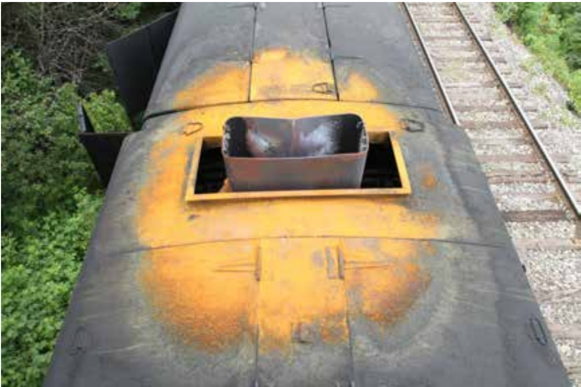
Figure 2: Rust showing where fire was concentrated around the cracked exhaust stack
