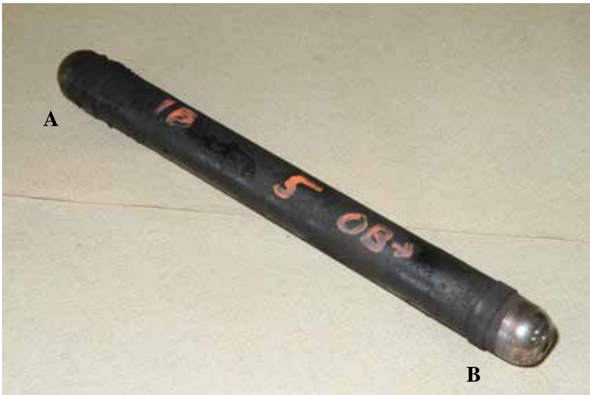
Figure 15: Exhaust crossover pushrod from PA 5 Inboard (A) and outboard (B) ends are labelled
