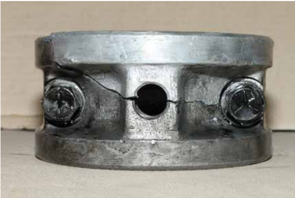
Figure 41: External view of subject cam bearing showing location of fracture
