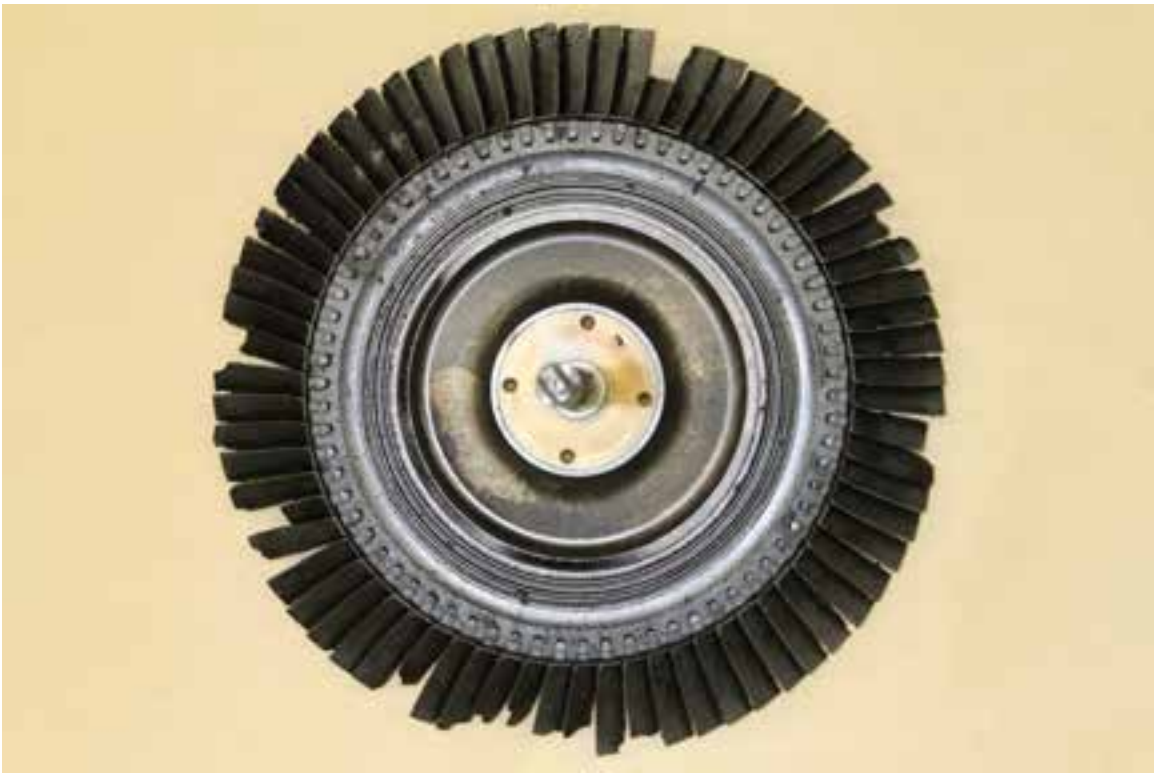
Figure 29: Damaged turbine blades
