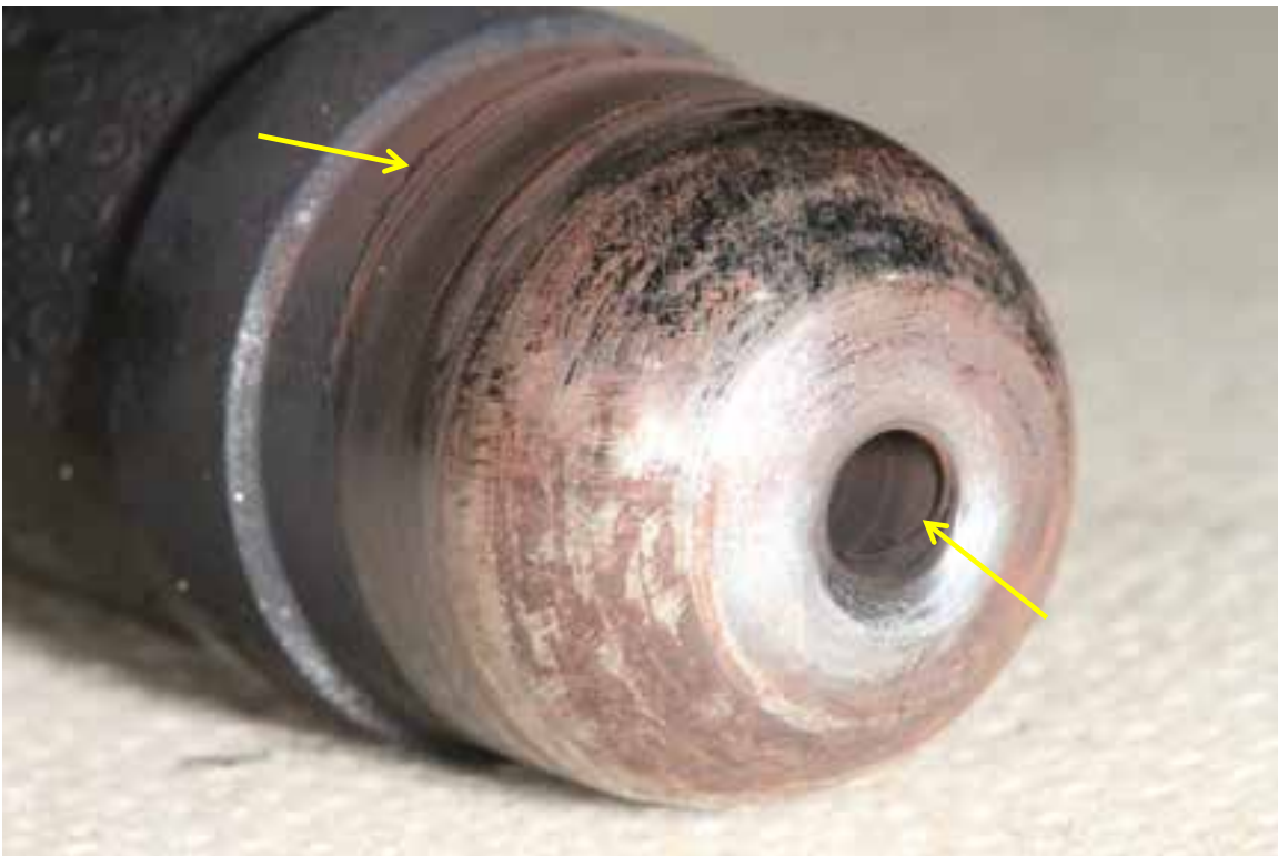
Figure 16: Close-up of outboard end of the exhaust crossover pushrod from PA 5 Fretting damage is visible (arrowed)
