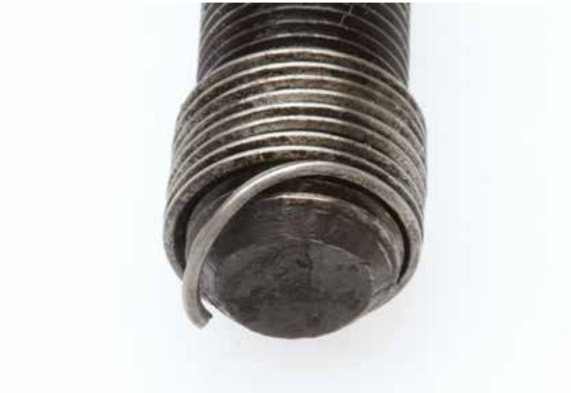
Figure 48: Axial deformation of the thread insert
