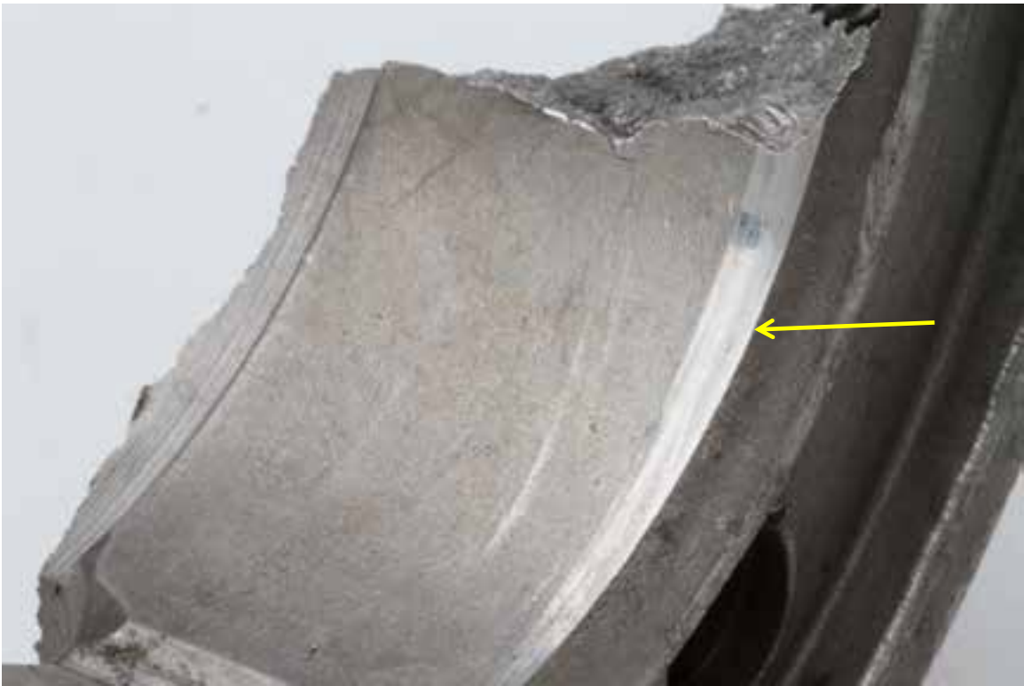
Figure 49: Smear on outboard edge of separated cam bearing portion (arrowed)
