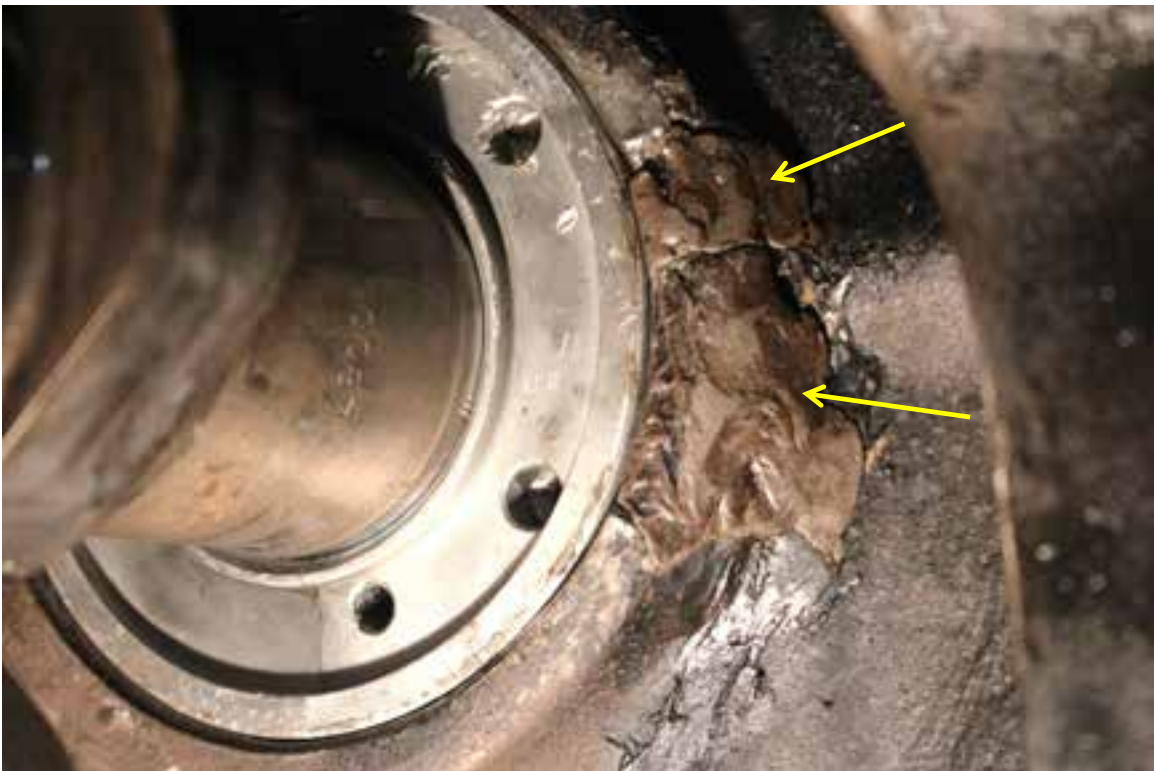
Figure 40: Recovered polymeric material pieces refitted showing extent of repair (arrowed)
