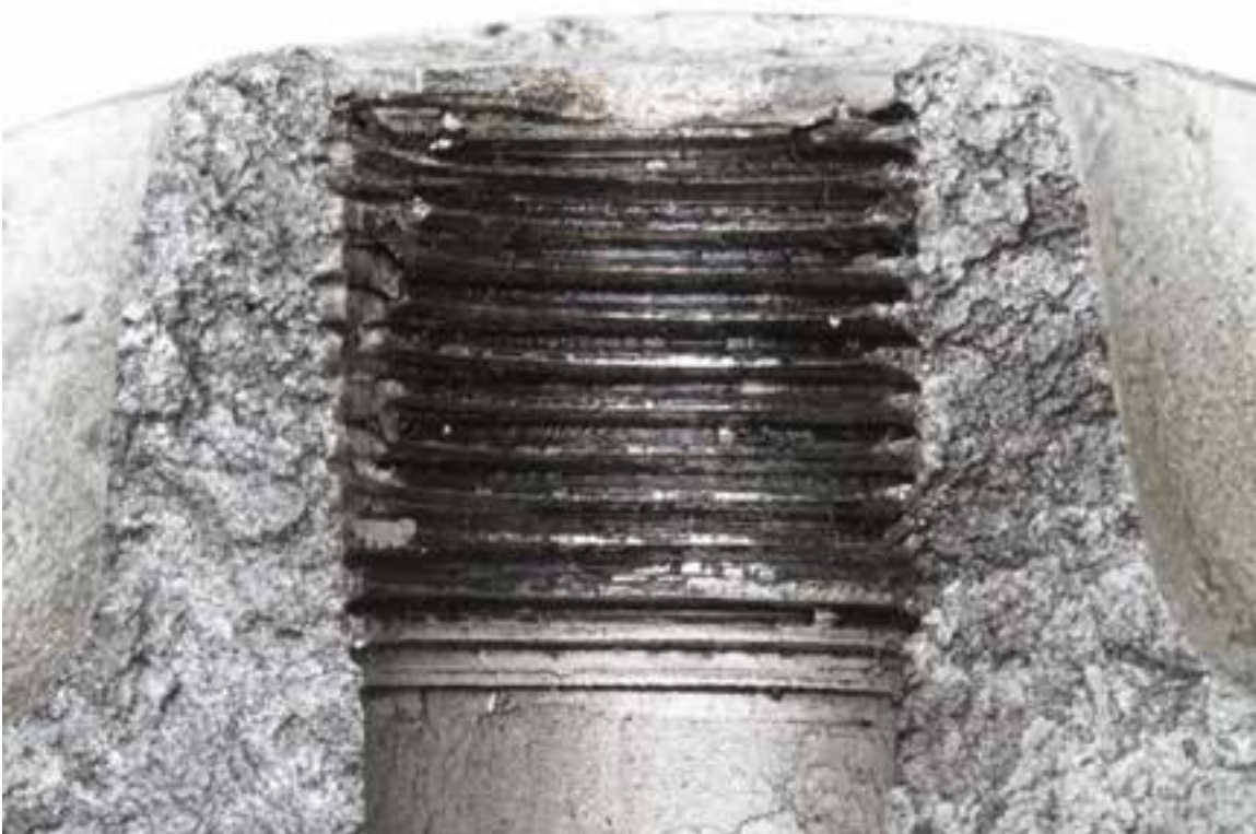
Figure 46: Mounting bolt thread damage in remaining portion of cam bearing Note the thread damage is localized at the fracture edges
