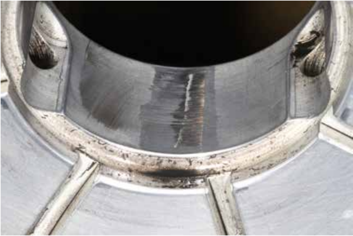
Figure 33: Close-up of turbine bearing damage
