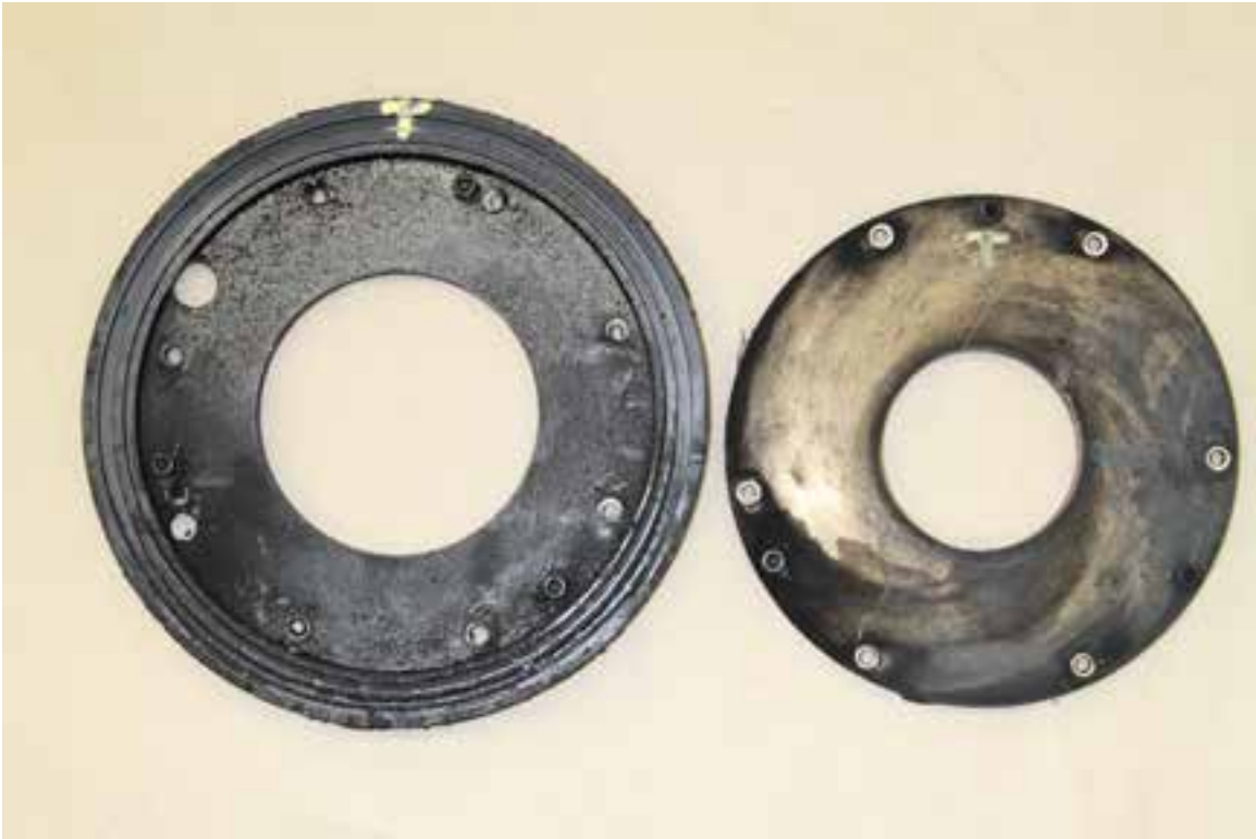
Figure 35: Turbine and compressor bearing oil seals
