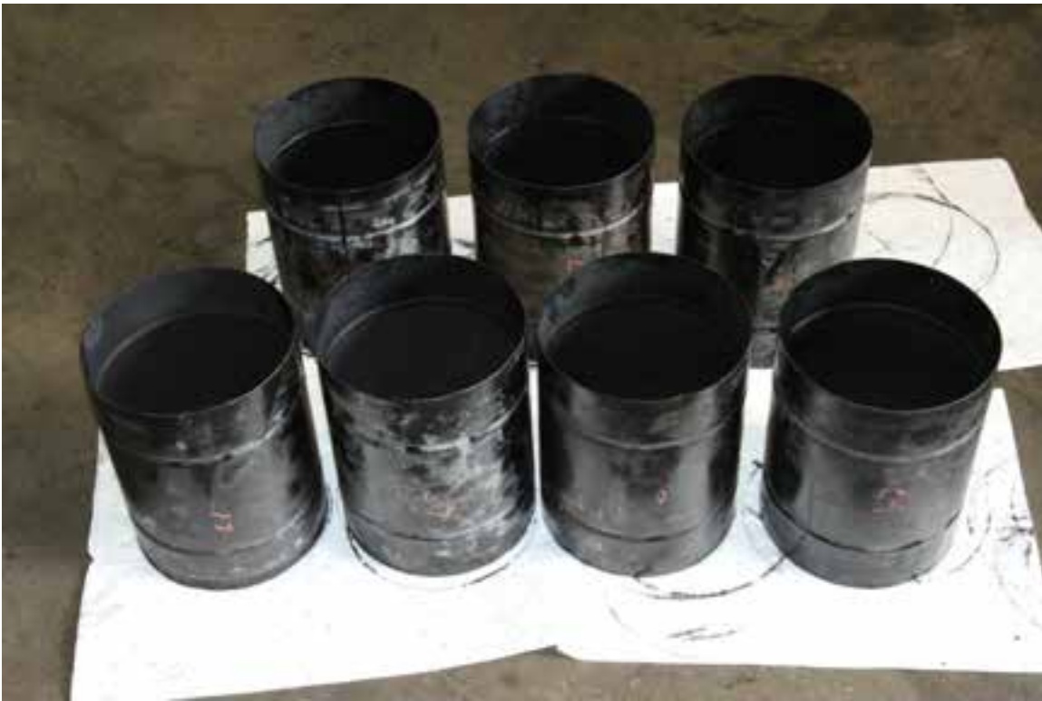
Figure 9: Left side intake manifold tube sections showing oil buildup
