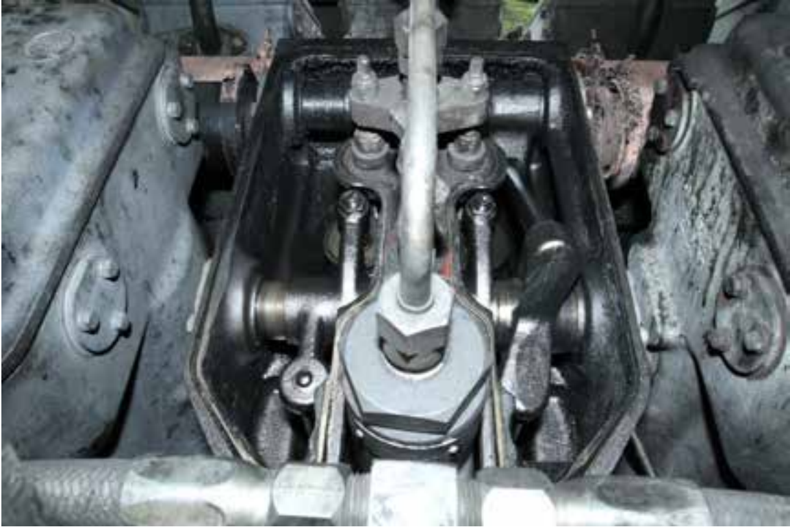
Figure 5: Normal oily valve train shown for comparison
