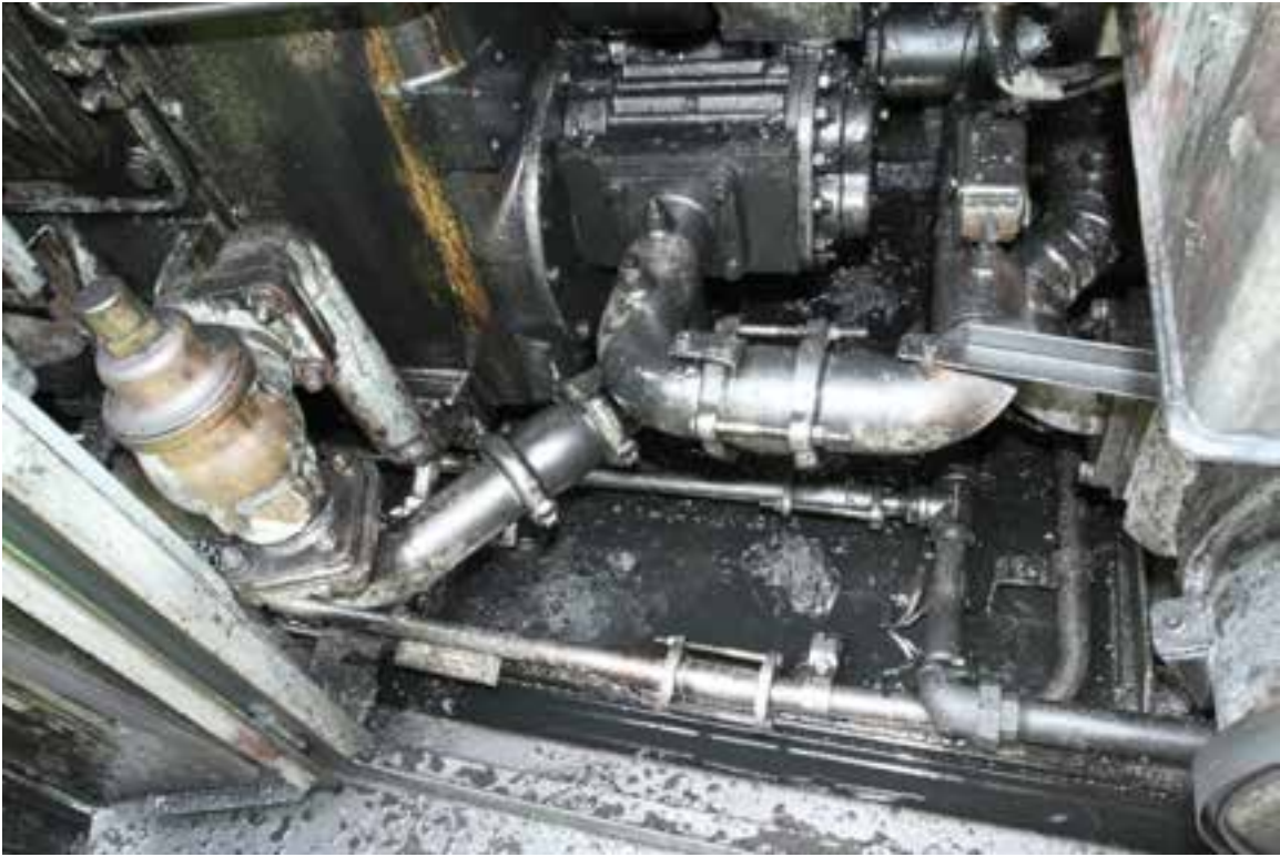
Figure 1: Representative view of engine oil dispersed inside MMA 5017 engine bay
