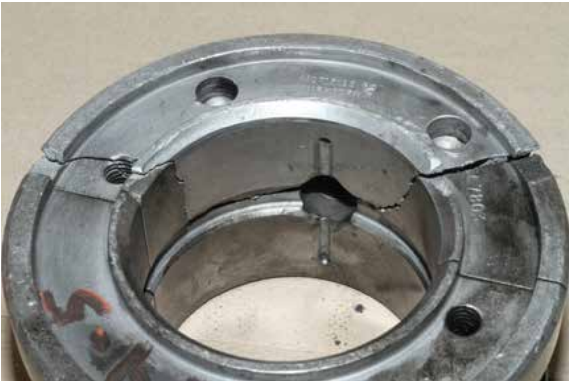
Figure 42: Internal view of subject cam bearing showing location of fracture
