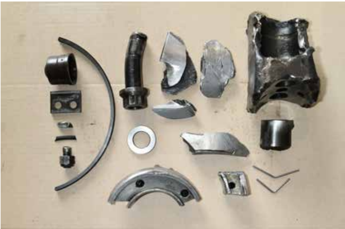
Figure 38: Debris recovered from MMA 5017 engine oil sump
