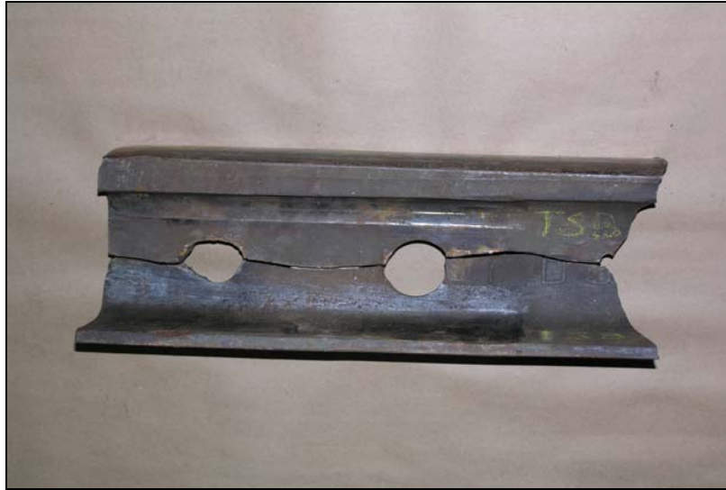
Photo 2. Fracture through the bolt holes
