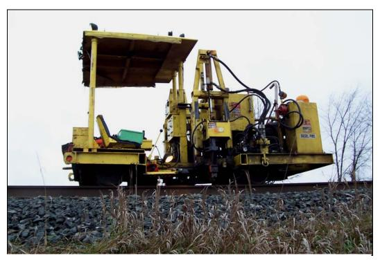
**Photo 1**. Side view of spike puller at accident location (*Source: OMOL*).
