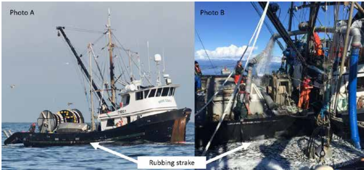
Figure 3. The rubbing strake on the Miss Cory , shown above the surface of the water while the vessel is voyaging (Photo A) and submerged while the vessel lists during operations (Photo B)
