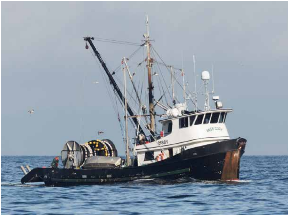
Figure 1. The Miss Cory in November 2016, outfitted for salmon purse seining (Source: Randy Hall, photographer)
