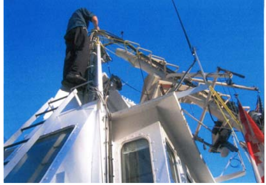
Photo 6. Damaged mast and radar assembly on Petite Forte
