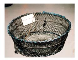
Concerned about conservation and sustainability in the prawn industry stemming from inappropriate use of the older bucket-type prawn traps, DFO set the upper limits for traps by volume and mesh size in 1995. The specifications were set at 170 litre volume and 38.1 mm mesh size, but no consideration was given to the weight of the traps. When licence holders acted to make their traps more robust and keep their volumetric shape and size, the weight of traps increased from 2 kg to 5 kg.
