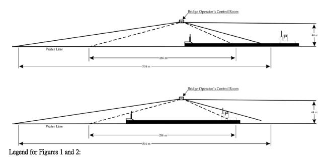
The area within the straight lines (i.e. ——) represents the lower limit when the operator is seated at the control panel.
