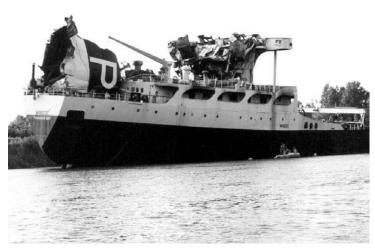
engine room casing and main engine were damaged by fire, heat and water. The bilge shell plating in way of starboard ballast tank No. 1 was creased and fractured. The aft bulkhead and bilge floors were distorted and torn adrift. The vessel was declared a constructive total loss. No damage to the cargo was reported (see Photo 4).
