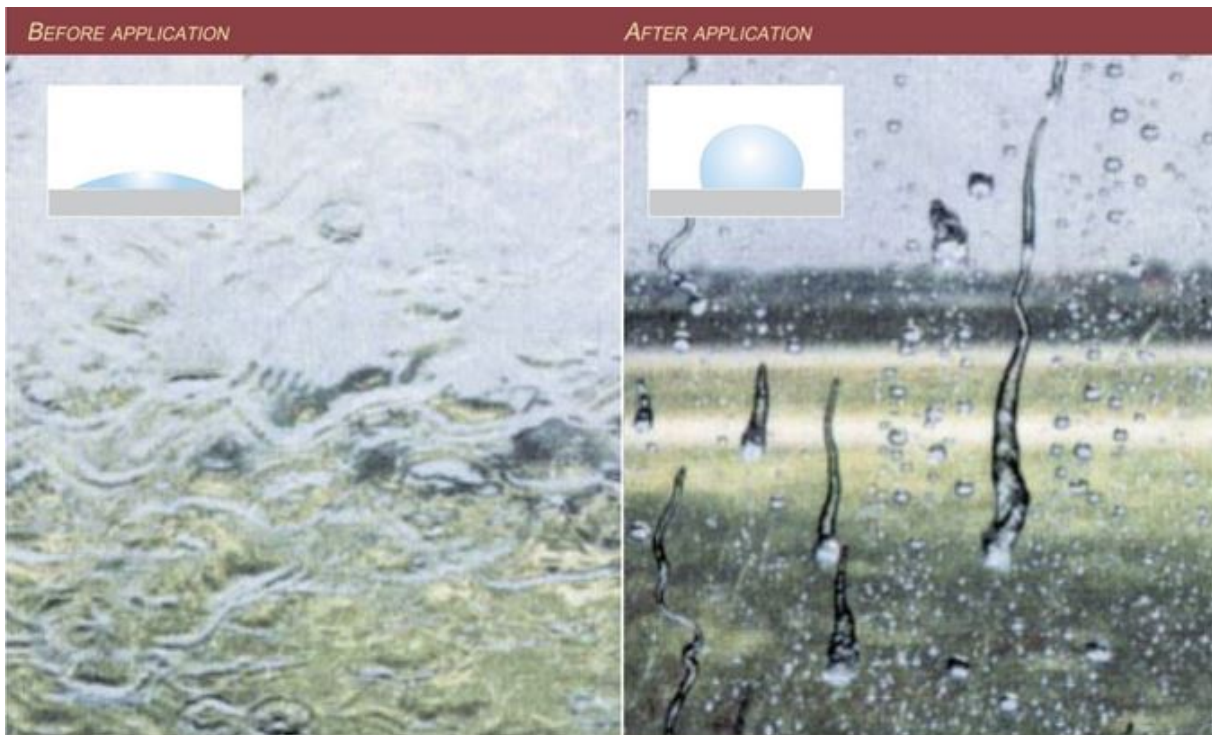
Figure 3. Illustration of the general effects of rain repellent at point of contact between drops of water and a windshield. (Source: Airbus Industrie, FAST – Airbus Technical Digest , Number 23 [October 1998], "Combining Environment Protection and Windshield Rain Protection on Airbus Aircraft", p. 23)
