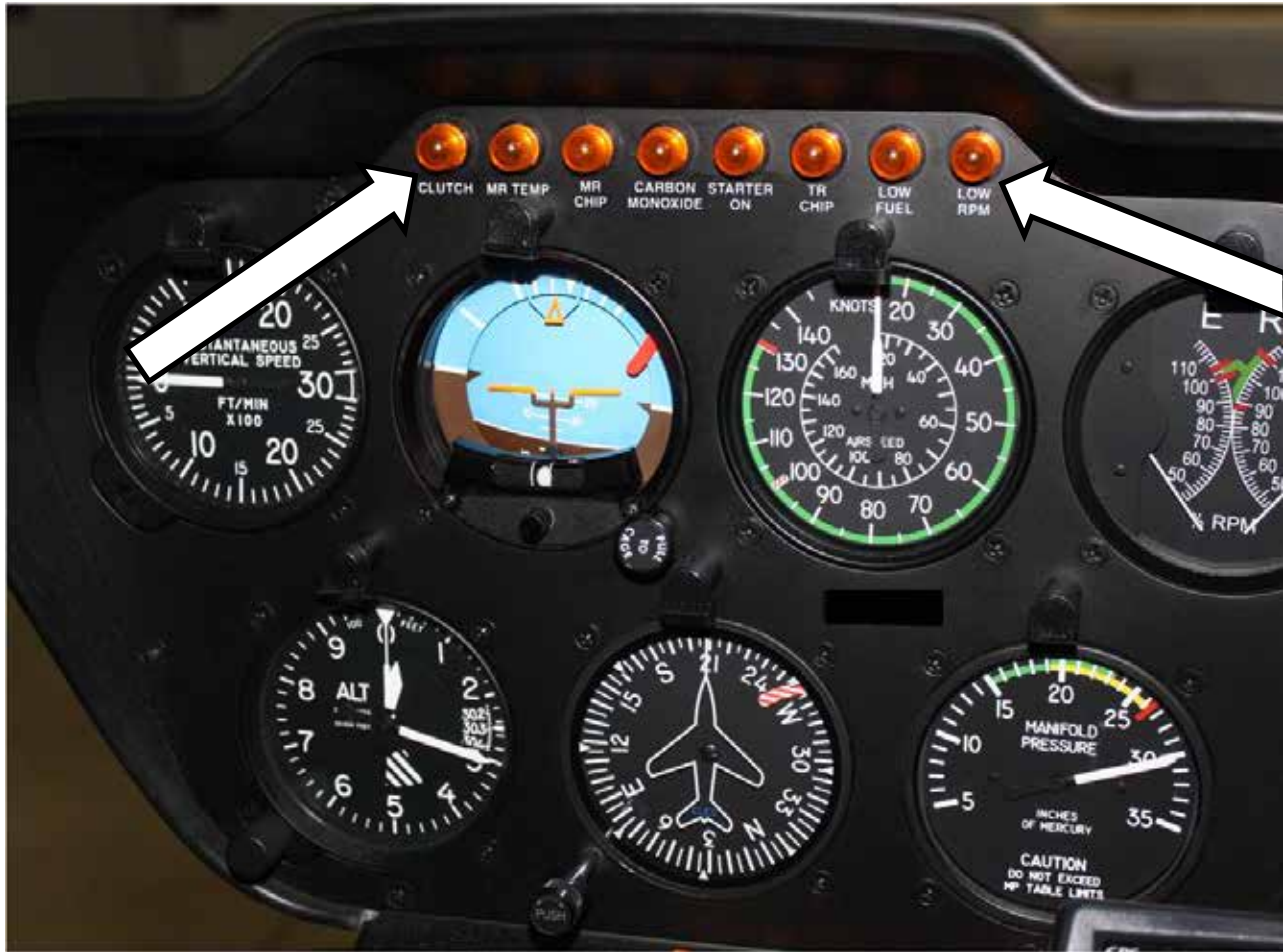
Photo 2. Instrument panel of a typical R44
