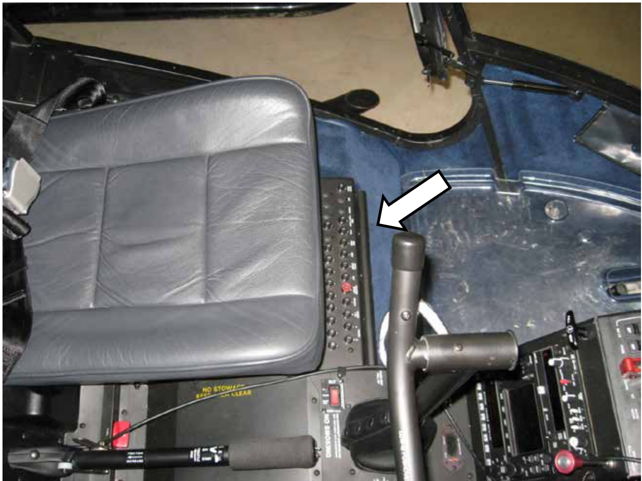
Photo 4. Left breaker panel
