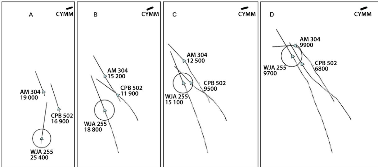
The circle around WJA 255 represents five nautical miles. The projected track lines for each aircraft represents three minutes and the altitudes are in feet above sea level. The letters A, B, C, and D correspond to the areas identified on the descent profile in Appendix B.
