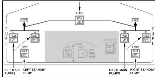
Figure 4. Fuel system controls
