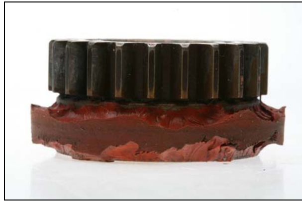
Photo 1. Gear damage to rubber material
