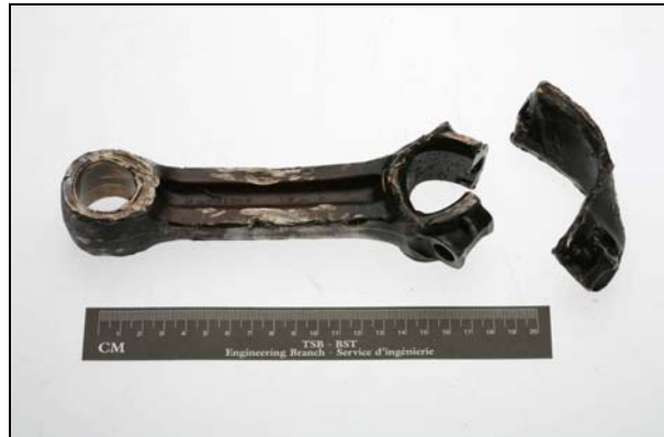
Photo 2. Heat and contact damage to connecting rod 2
