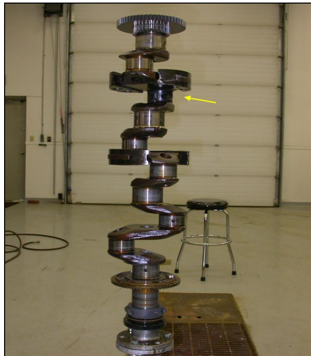
Photo 3. Crankshaft showing heated area
