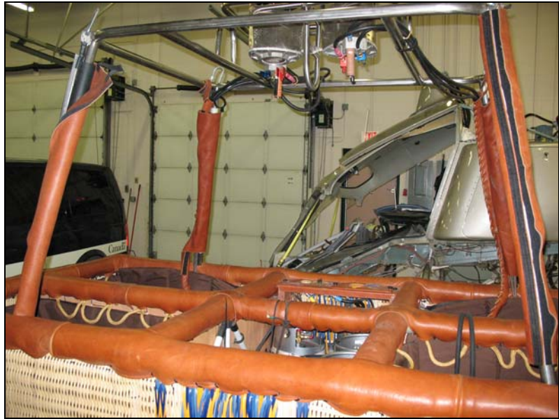
Photo 2. Example of basket and burner frame assembly
