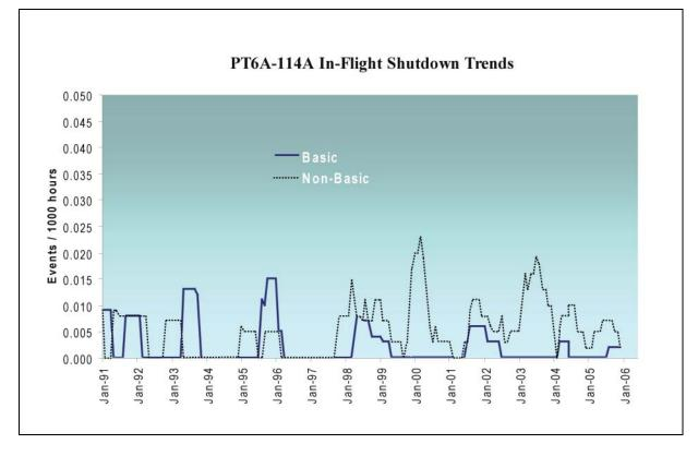
A basic In Flight Shut Down (IFSD) is an IFSD caused by a malfunction directly related to the engine or an engine component (solid line). These events are used in mean time before failure (MTBF) calculations and include unsubstantiated events where investigations are still in progress to identify the primary part that caused the event.
