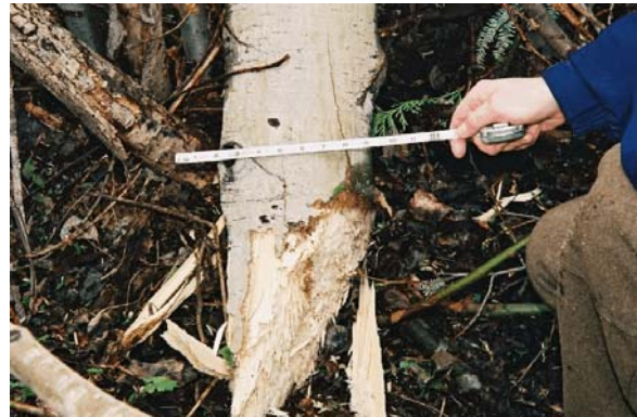
Figure 4. 7 1/2" diameter tree cut by main rotor blade
